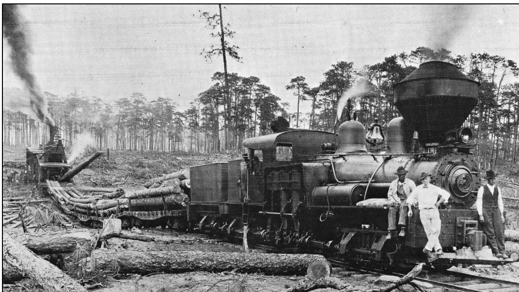
This photo illustrates the efficiency of the logging operation and the problem created by it. The log cars are being loaded by a steam-powered log loader and no forest remains to provide for natural regeneration (from Taber 1971).
