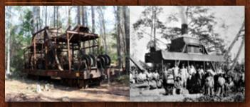
logging equipment. The skidder operated on the track and at one setting with four cables extending out, trees could be harvested from 40 acres. It was a massive machine and its operation resulted in complete destruction of vegetation on the harvest site. This is the only Clyde skidder now known to exist.
