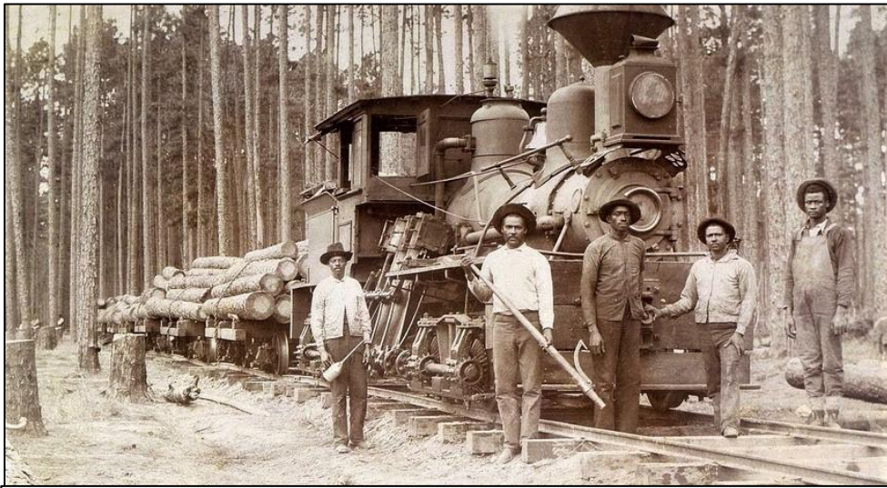
Crowell and Spencer locomotive #1 was a Shay Patent geared engine, built in 1895 by the Lima Locomotive Works of Lima, OH. Stamps Crowell took this photo southwest of Long Leaf, LA, in about 1895 with his new Brownie Box camera. (Stamps Crowell photo, Crowell Family Collection, Southern Forest Heritage Museum)
