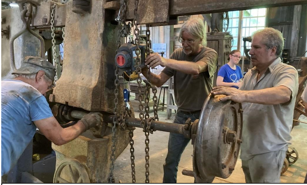
Volunteers Michael Brown, Mike Miller, and Glen Armand use the hydraulic wheel press to remove a wheel from the axle of the Museum's M-4 Rail Passenger Car. (Photo by Jason Rose)
