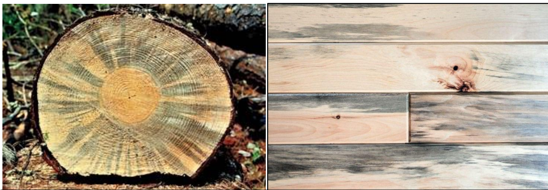
Cross section of southern pine beetle killed southern pine showing the development of blue stain in the sapwood (left, photo from Richard F. Billings, Texas A&M Forest Service) and, right, lumber infested with the blue-stain fungus.
